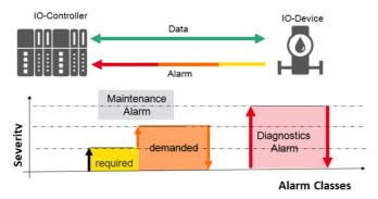
Fig. 7: PROFINET diagnosis model for signaling faults with different priority
