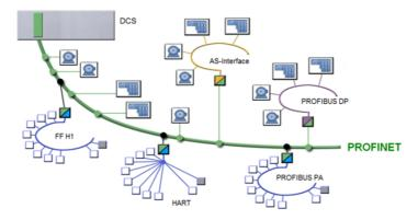
Fig. 14: Investment protection through integration of plant units using proxies
