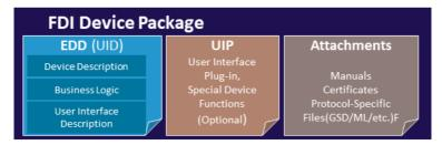
Fig. 17: The FDI technology building blocks
