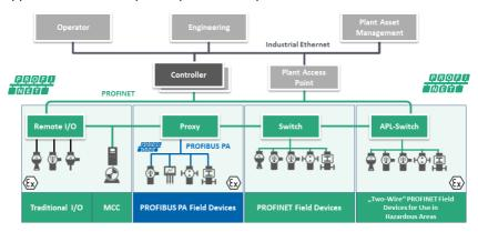
Fig. 3: PROFINET and PROFIBUS PA, and in the future with APL
