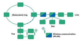
Fig. 4: Flexible network configuration of PROFINET
