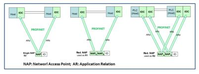
Fig. 13: System redundancy
