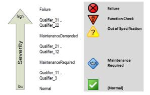
Fig. 8: Assignment of the PROFINET device diagnostics to NAMUR NE 107 requirements
