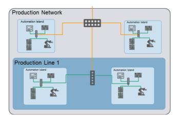
Fig. 10: Segmentation of the network
