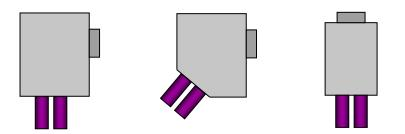
Figure 3-10: Design variants of Sub-D connectors
