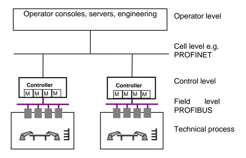
Figure 1-2: Using PROFIBUS in process automation
