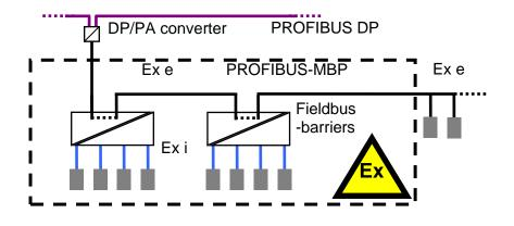
Figure 3-19: Fieldbus barriers for PROFIBUS-MBP (PA)
