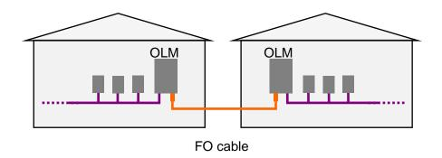
Figure 3-35: Application of FO technology for the connection of buildings
