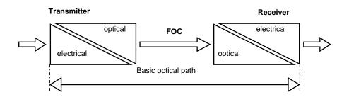
Figure 3-36: Basic optical path
