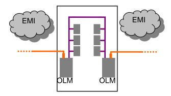
Figure 3-34: Application of FO technology for connection of cabinet with EMI
