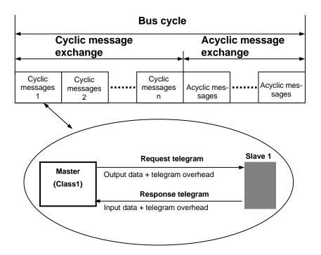
Figure 2-10: Basic structure of a bus cycle
