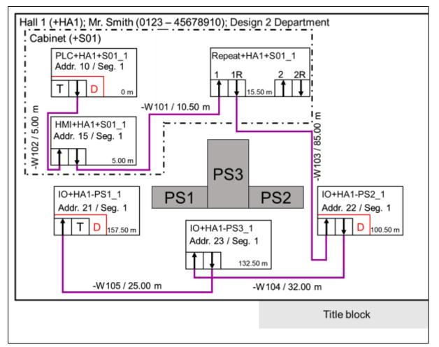
Figure 5-4: Example of PROFIBUS forwards documentation, physical topology plan
