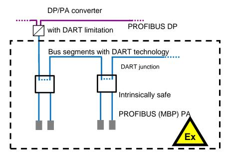
Figure 3-29: Intrinsically safe topology with trunk and spur and high power
