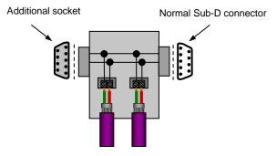
Figure 3-9: Sub-D connector with additional socket
