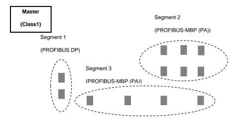
Figure 2-4: Segment forming using node groups
