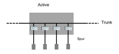
Figure 3-26: Example of an active junction module, non-Ex
