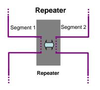
Figure 2-6: Connecting two segments to a repeater
