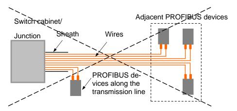
Figure 3-41: Problem when stripping break-out cables
