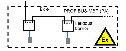
Figure 3-27: Spur coupler in hazardous area
