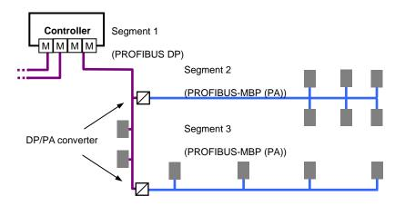
Figure 2-3 shows a possible setup of a network to provide an overview
