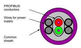
Figure 3-6: Structure of a hybrid cable
