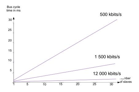
Figure 2-11: PROFIBUS DP bus cycle times
