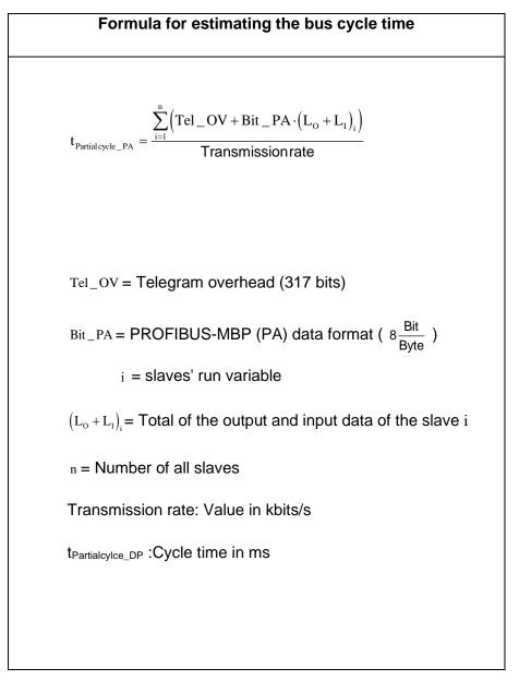
Figure 2-12 provides a graphical representation of the formula shown in Table 2-7 for the fixed transmission rate of 31.25 kbit/s for PROFIBUS-MBP (PA). The bus cycle times for PROFIBUS DP are shown in the same graphic as a reference. Again, it is assumed that each slave uses 5 bytes of input and output data.
