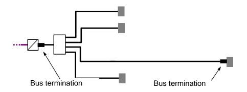
Figure 3-31: Alternative installation of bus terminations for PROFIBUS-MBP (PA)
