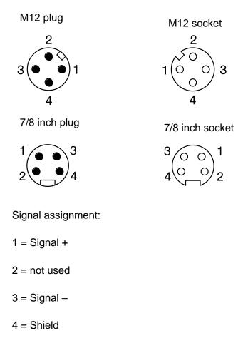
Figure 3-24: Pin assignment of M12 and 7/8 inch plug and socket connectors
