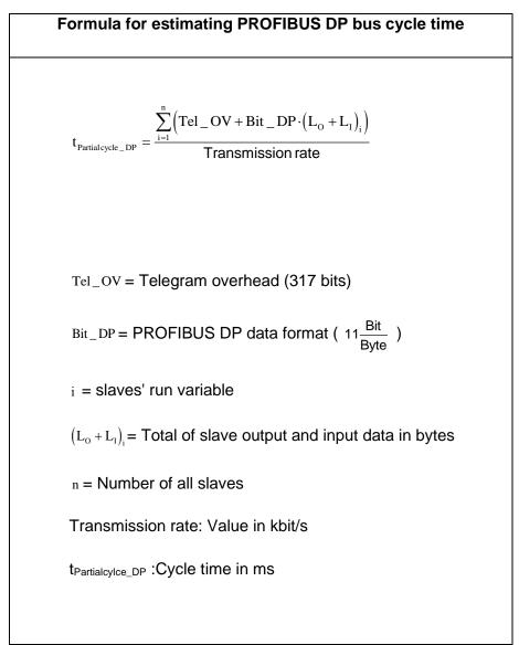
Figure 2-11 provides a graphical overview of the formula shown in Table 2-6 for various transmission rates. It is assumed that each slave uses 5 bytes of input and output data. This calculation rather represents a particularly favorable case, as no reserves for the repetition of corrupted messages and acyclic communication for masters Class 2 is taken into account.
