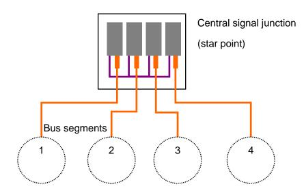
Figure 3-37: Star topology using OLMs
