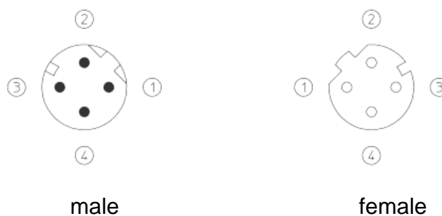
Figure 9.3.3.1-2: M12 D-coded contact assignment and coding
